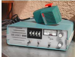
Mobil-FM-Transceiver SE 280, 144-146 MHz in 80 Kanälen
