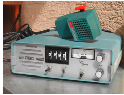
Mobil-FM-Transceiver SE 280, 144-146 MHz in 80 Kanälen
