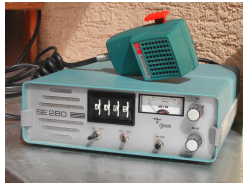
Mobil-FM-Transceiver SE 280, 144-146 MHz in 80 Kanälen
