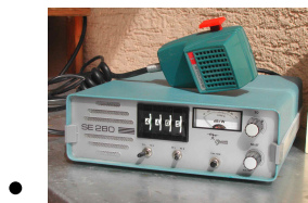
Mobil-FM-Transceiver SE 280, 144-146 MHz in 80 Kanälen
