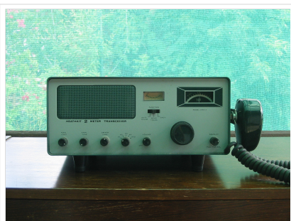
Heathkit HW17 2m AM Transceiver
