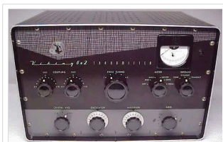
6m/2m Sender ab 1957, Power: AM 50 W, CW 80 W
