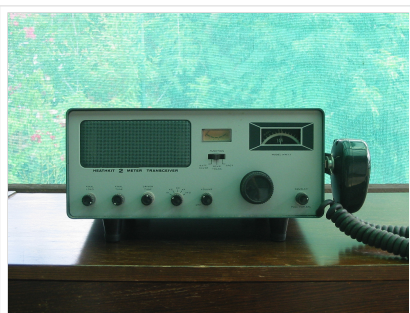
Heathkit HW17 2m AM Transceiver
