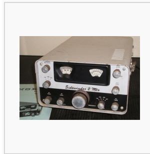
Gonset 2M Sidewinder CW/SSB /AM transceiver, Modell 900A
