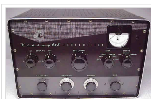
6m/2m Sender ab 1957, Power: AM 50 W, CW 80 W
