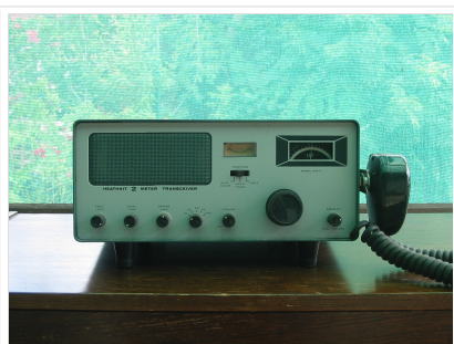
Heathkit HW17 2m AM Transceiver
